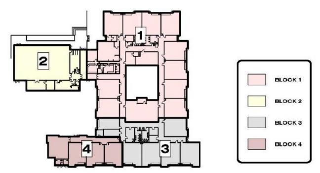
Major upgrade items include the refastening of the existing steel decking, deck to wall connections throughout the whole school, drag struts to the top of the deck in Block 3, and replacement of roofing. The construction started in September of 2021, with completion in Mid-February 2023. Two weeks were recently lost to the schedule due the inability to roof during extreme low temperatures and the snow build up in December 2022.
